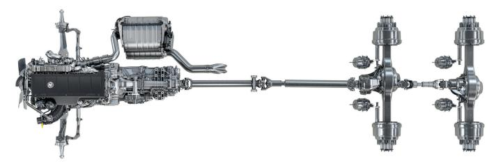
The DT12<sup>®</sup> transmission links engines to axles and communicates with the DD13<sup>®</sup> Gen 5 and DD15<sup>®</sup> Gen 5 on an integrated electronics network to share damage-reducing information such as clutch overloading and driveline protection.
