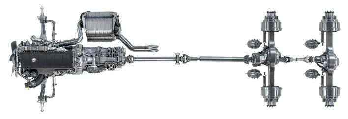
The DT12<sup>®</sup> transmission links engines to axles and communicates with the DD13<sup>®</sup> Gen 5 and DD15<sup>®</sup> Gen 5 on an integrated electronics network to share damage-reducing information such as clutch overloading and driveline protection.
